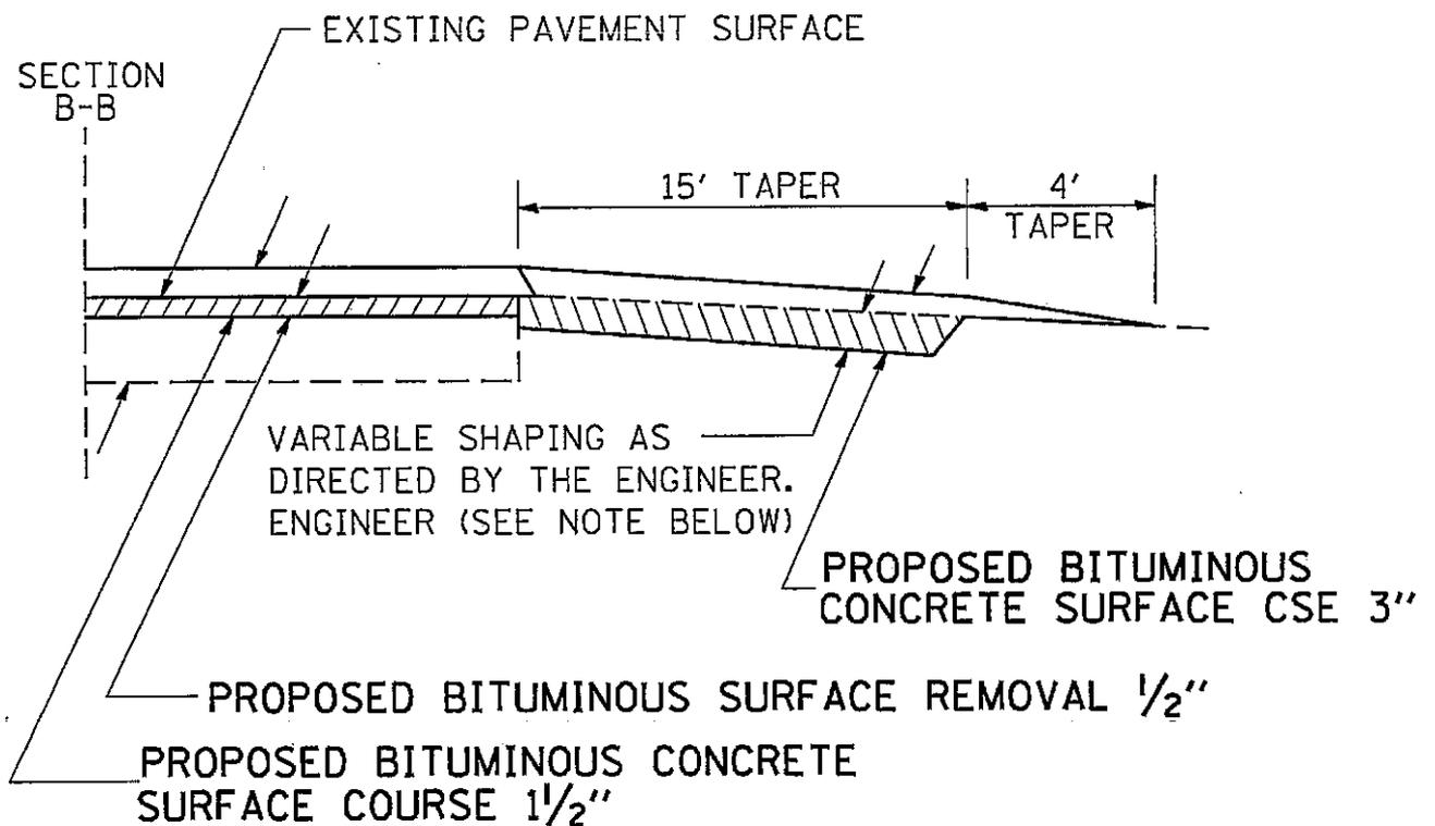
IF EXISTING SUB-BASE IS INADEQUATE, AS DETERMINED BY THE ENGINEER, THE SIDEROADS SHALL BE CORED OUT AND AGGREGATE SUB-BASE, TYPE B SHALL BE PLACED FOR BASE. THE COST OF CORING OUT THE SIDEROAD SHALL BE INCLUDED IN THE COST OF THE AGGREGATE BASE COURSE. IF EXISTING SUB-BASE IS DETERMINED TO BE ADEQUATE, THE AGGREGATE BASE COURSE SHALL BE DELETED AND THE PREPARATION OF THE BASE SHALL BE CONSTRUCTED ACCORDING TO ARTICLE 406.09
