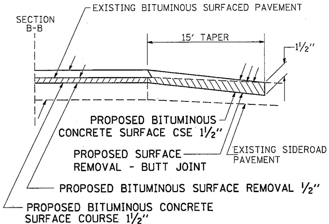
IF EXISTING BASE COURSE IS INADEQUATE, AS DETERMINED BY THE ENGINEER, THE SIDEROADS SHALL BE CORED OUT AND AGGREGATE BASE COURSE, TYPE B SHALL BE PLACED FOR BASE. THE COST OF CORING OUT THE SIDEROAD SHALL BE INCLUDED IN THE COST OF THE AGGREGATE BASE COURSE. IF EXISTING BASE COURSE IS DETERMINED TO BE ADEQUATE, THE AGGREGATE BASE COURSE SHALL BE DELETED AND THE PREPARATION OF THE BASE SHALL BE CONSTRUCTED ACCORDING TO ARTICLE 406.09.
