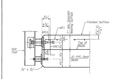
RAIL ANCHOR DEVICE DETAIL
