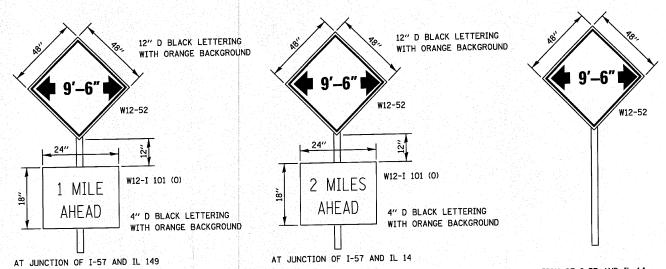
A W12-52 SIGN. WITH A W12-I101 SIGN, SHALL BE ERECTED AT THE JUNCTION OF I-57 AND IL 149 AND AT THE JUNCTION OF I-57 AND IL 14. THE ACTUAL LOCATION OF THE SIGNS TO BE DETERMINED BY THE ENGINEER. AN ADDITIONAL W12-52 SIGN SHALL BE ERECTED 1000 FEET IN EACH DIRECTION FROM THE INTERCHANGE PRIOR TO STAGE 1 CONSTRUCTION. THESE SIGNS SHALL BE MAINTAINED BY THE CONTRACTOR DURING STAGE CONSTRUCTION AND SHALL BE REMOVED AT THE COMPLETION OF ALL STAGED CONSTRUCTION.
