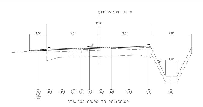
NOTE: IN AREAS OF SUPERELEVATION, PROPOSED PAVEMENT SURFACE MATCHES EXISTING SUPERELEVATION
