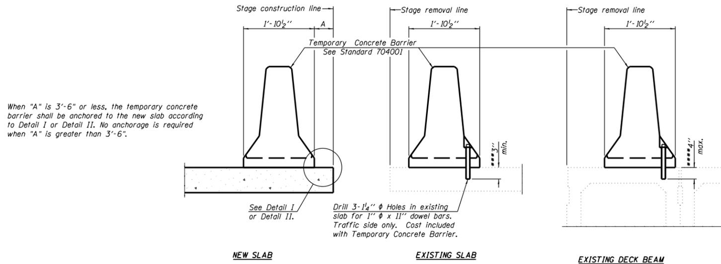
When "A" is 3'-6" or less, the temporary concrete barrier shall be anchored to the new slab according to Detail I or Detail II. No anchorage is required when "A" is greater than 3'-6".
