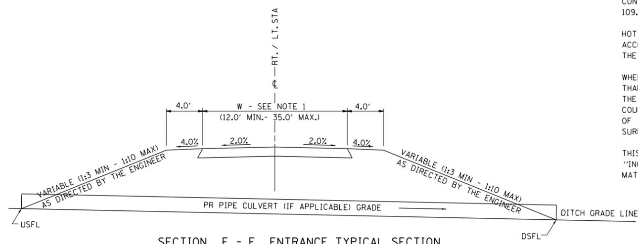
NOTE 1: WIDTH OF ENTRANCE MAY BE INCREASED AT THE PIPE CULVERT DUE TO THE DITCHLINE BEING LOCATED IN THE ENTRANCE FLARE AREA.
