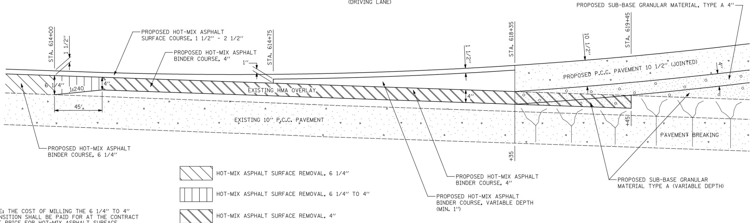
NOTE: THE COST OF MILLING THE 6 1/4" TO 4" TRANSITION SHALL BE PAID FOR AT THE CONTRACT UNIT PRICE FOR HOT-MIX ASPHALT SURFACE REMOVAL 6 1/4" AND NO ADDITIONAL COMPENSATION SHALL BE ALLOWED.
