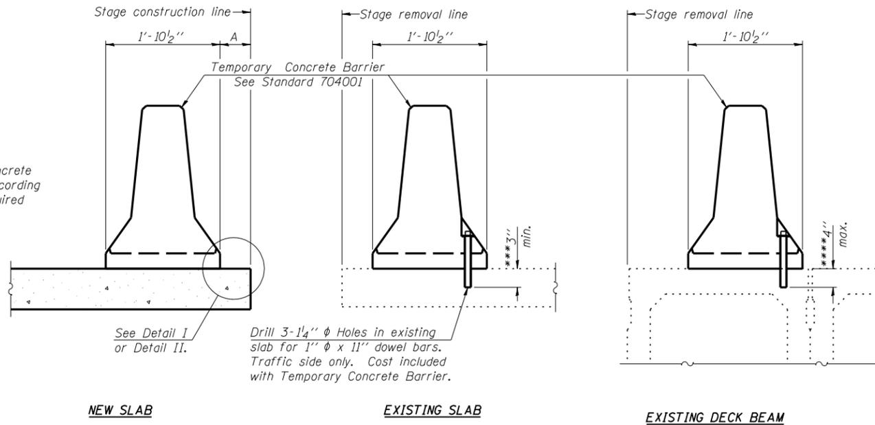
Drill 3-1/4"  $\phi$  Holes in existing slab for 1"  $\phi$  x 11" dowel bars. Traffic side only. Cost included with Temporary Concrete Barrier.
