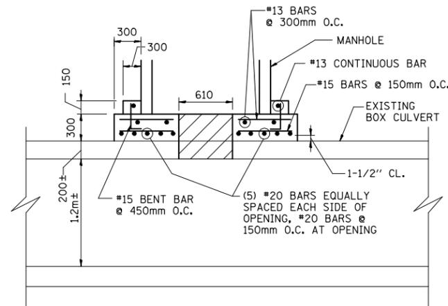
**STORM SEWER MANHOLE DETAIL ON EXISTING STRUCTURE 057-8029**
