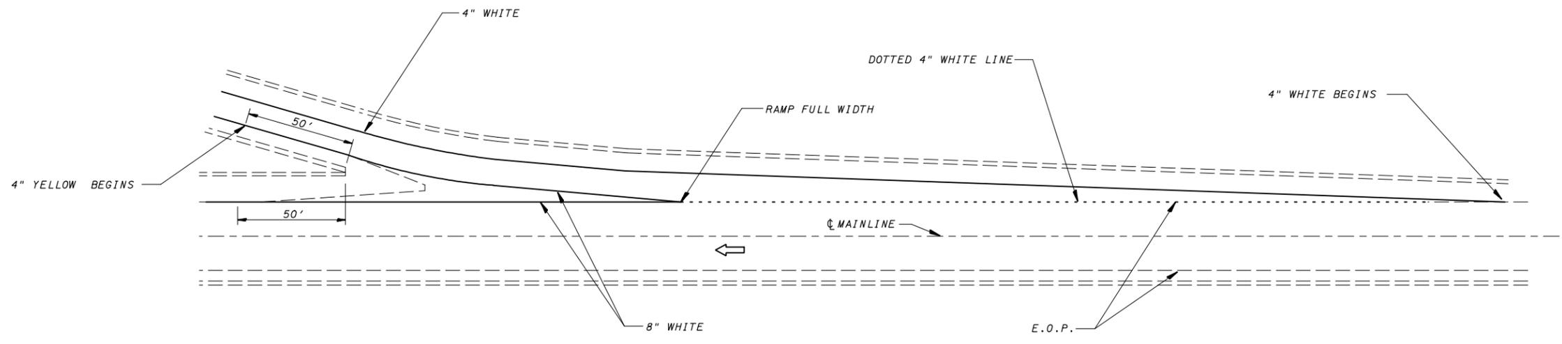
**TYPICAL PAVEMENT MARKINGS FOR EXIT RAMP TERMINALS**
