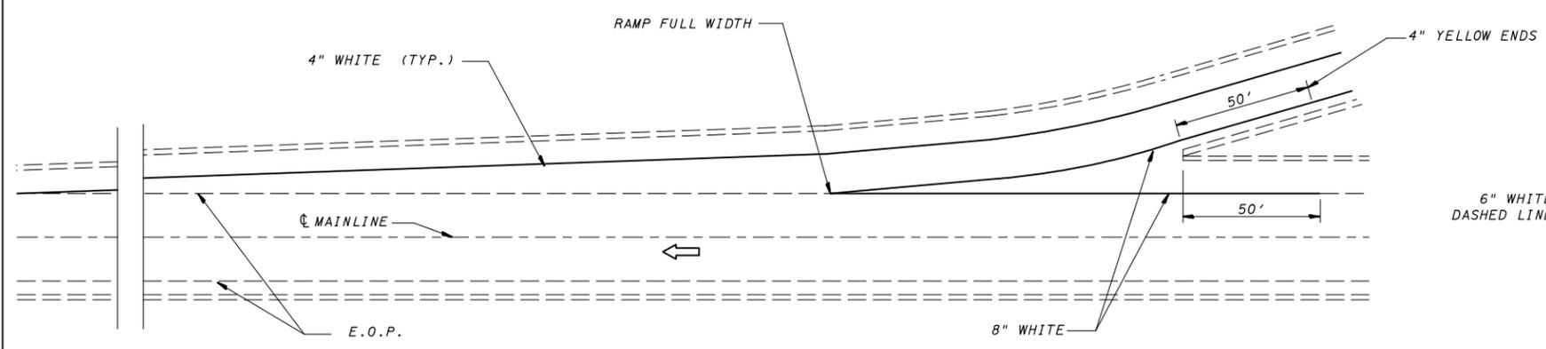
**TYPICAL PAVEMENT MARKING FOR ENTRANCE RAMP TERMINALS**
