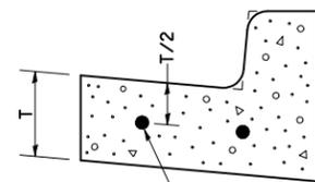
CONTINUOUSLY REINFORCED WITH 2 - \*15 BARS EVENLY SPACED
