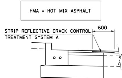
**DETAIL OF PROPOSED STRIP REFLECTIVE CRACK CONTROL TREATMENT**
