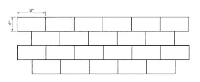
STAMPED CONCRETE IN A 4" X 8" RUNNING BOND PATTERN, BRICK RED COLOR WITH CHARCOAL RELEASE AGENT TO MATCH COLOR AND PATTERN CURRENTLY IN USE IN UTICA CROSSWALKS. SEE SHEETS 77-79 FOR LAYOUT AND DIMENSIONS OF CROSSWALKS.
