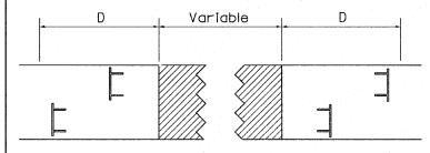
Type III Barricades and R11-4-4830 signs shall be as shown in "Road Closed To All Thru Traffic" detail on Highway Standard 701901. If the distance "D" exceeds 600 m (2000') an additional set of barricades and R11-4-4830 shall be placed at each end of the work area.
