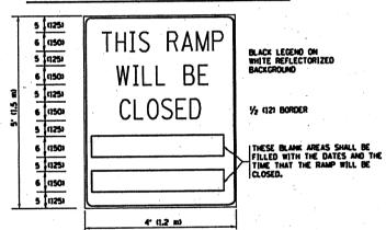
THESE SIGNS ARE REQUIRED ON BOTH SIDES OF THE RAMP, MINIMUM OF I WEEK IN ADVANCE OF THE CLOSUFE.
