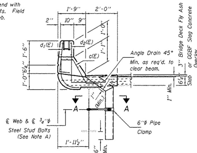
**SECTION THRU PARAPET AT EXISTING DRAIN**
