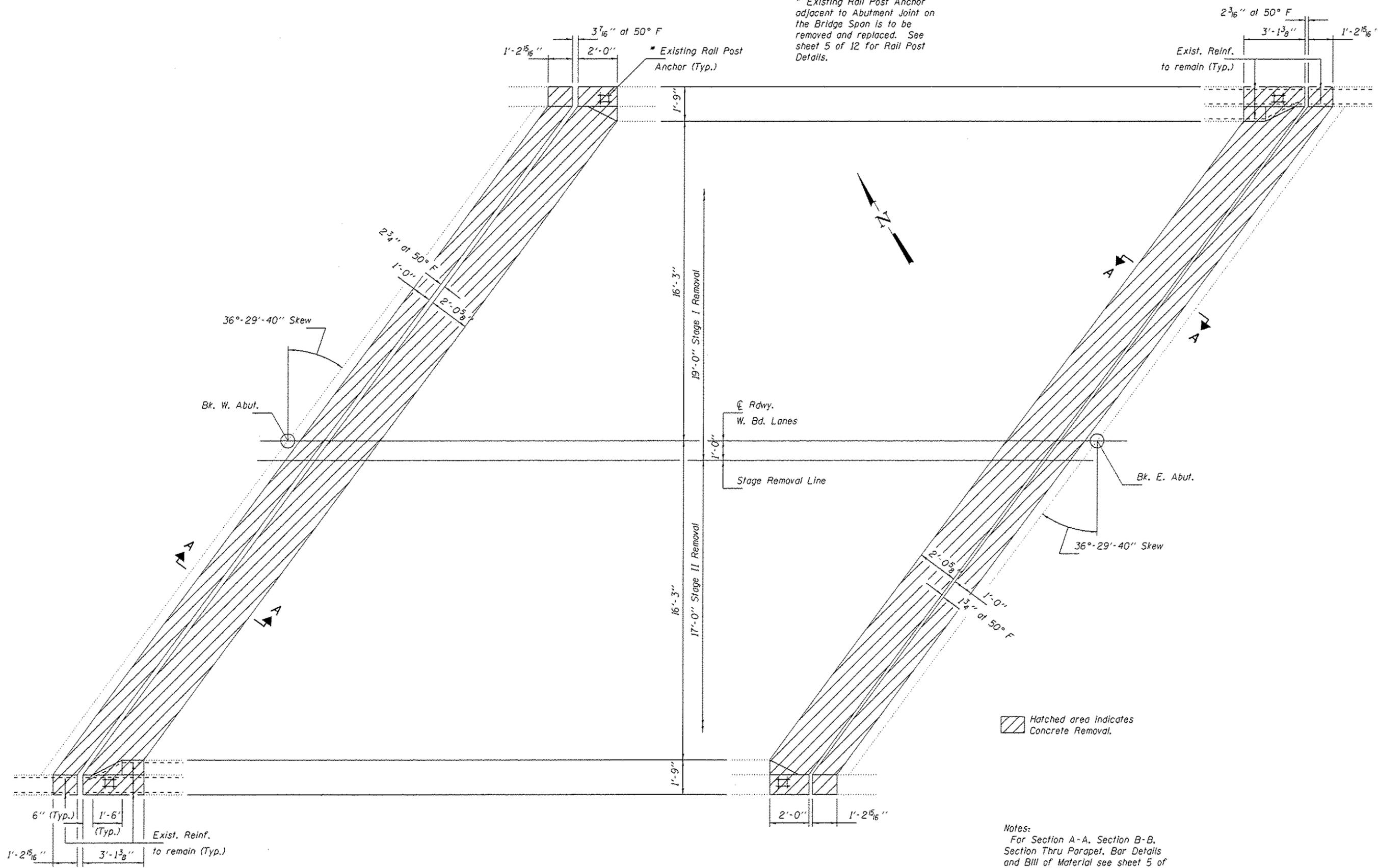
Hatched area indicates Concrete Removal.
