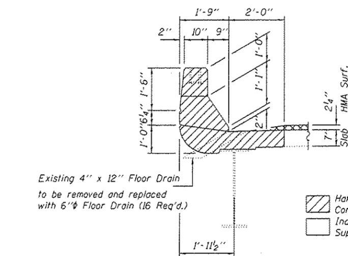
**SECTION THRU PARAPET AT EXISTING DRAIN**
