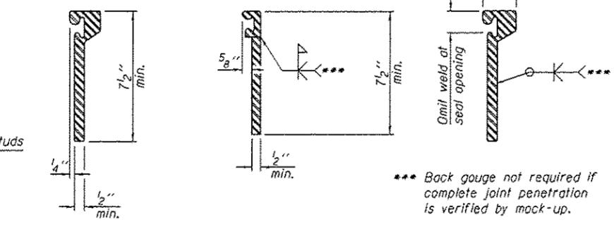
\*\*\* Back gouge not required if complete joint penetration is verified by mock-up.
