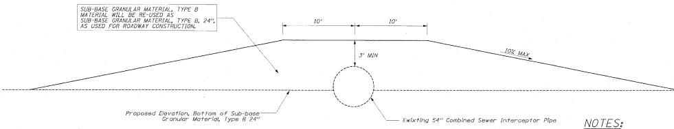
54" SEWER INTERCEPTOR (STA. 1385+44 SB, 2385+64 NB) 36" WATER MAIN (STA. 1533+28 SB, 2533+49 NB) CONSTRUCTION PROTECTION
