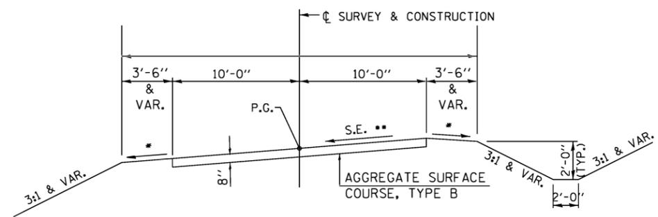
TYPICAL FILL SECTION CONSTRUCT AS SHOWN ON STATION CROSS SECTIONS.
