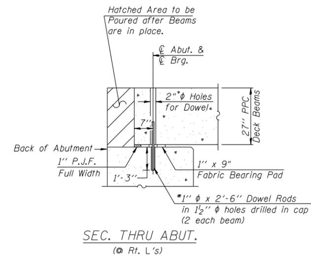
\* Note: After beams are in place, 1/2" holes shall be drilled into the Substructure, and the dowel rods grouted in place and allowed to cure (Min. 24 Hrs.) prior to grouting shear key.
