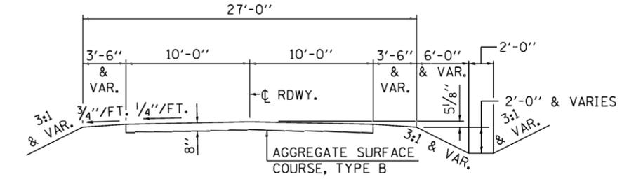
SUGGESTED FILL SECTION CONSTRUCT AS SHOWN BY STATION CROSS SECTIONS
