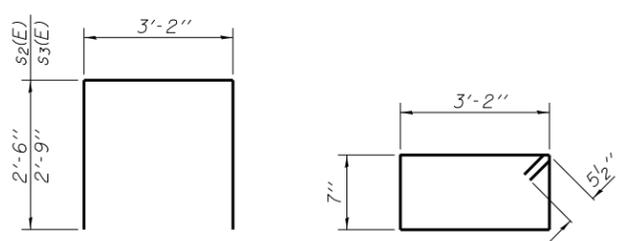
**BAR s<sub>2</sub>(E) & s<sub>3</sub>(E)**      **BAR s<sub>4</sub>(E)**
