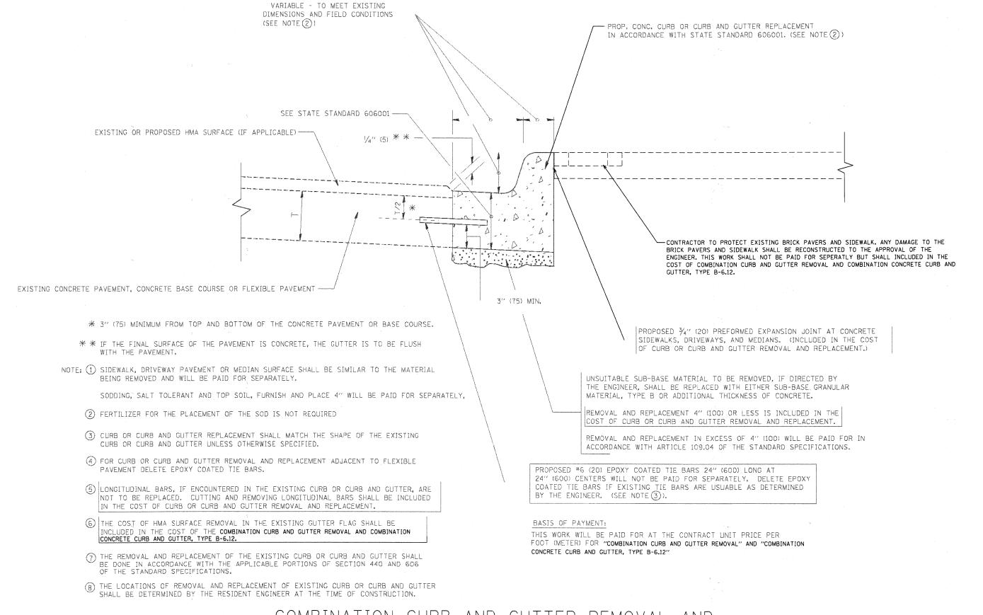
COMBINATION CURB AND GUTTER REMOVAL AND COMBINATION CONCRETE CURB AND
