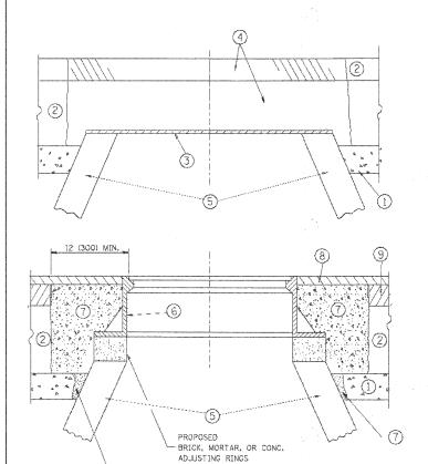
EXISTING BROKEN FRAMES AND LIDS SHALL BE REMOVED AND DISPOSED OF BY THE CONTRACTOR AND SHALL BE REPLACED AS DIRECTED BY THE ENGINEER, REPLACEMENT FRAMES AND LIDS WILL BE PAID FOR IN ACCORDANCE WITH ARTICLE 109.04 OF THE STANDARD SPECIFICATIONS UNLESS A SEPARATE PAY ITEM HAS BEEN PROVIDED.
