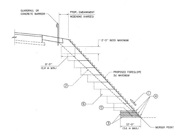
TYPICAL BENCHING DETAIL FOR EMBANKMENT
