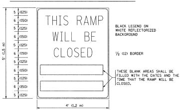
THESE SIGNS ARE REQUIRED ON BOTH SIDES OF THE RAMP, MINIMUM OF  $1\ \mbox{WEEK}$  IN ADVANCE OF THE CLOSURE.
