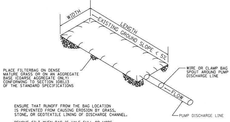
REMOVE SILT WHEN BAG IS HALF FULL OR MORE OFTEN IF RECOMMENDED BY THE MAUNFACUTURER. DISPOSE OF SILT BY TRANSPORTING THE FILLED BAG TO DISPOSAL AREA. SLIT THE BAG, BLEND SILT INTO EXISTING TOPOGRAPHY, SEED AND MULCH
