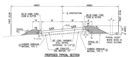
CARDINAL HILL RD. (C.H. 37) STA 517+37.86 - STA 525+57.88 S.E.A. STA 517+37.86 — STA 518+07.86 S.E.A. STA 524+89.93 — STA 526+99.93 SEE INTERSECTION DETAIL, SHEET 36: STA 525+89.93 — STA 528+75.45
