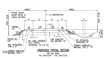
① 6-1/2" LOWER BINDER - 2 LIFTS 2-1/4" TOP LIFT BINDER (POLYMERIZED) 1-1/2" SURFACE LIFT (POLYMERIZED) [BITUMINOUS PRIME/RC 70 (FOG COAT) REQUIRED BETWEEN SUCESSIVE LIFTS]
