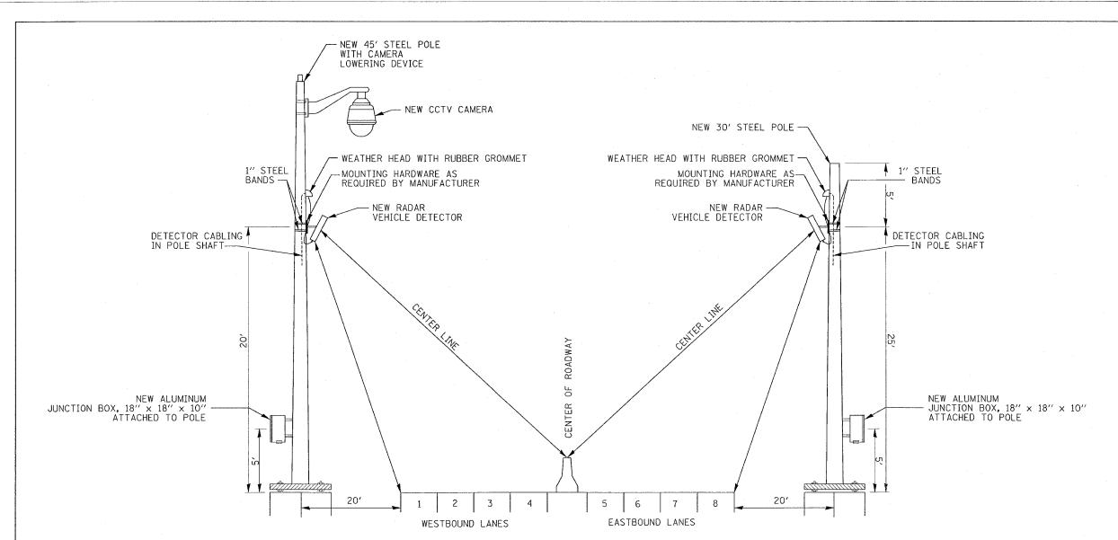
DETAIL RADAR VEHICLE DETECTOR NOT TO SCALE
