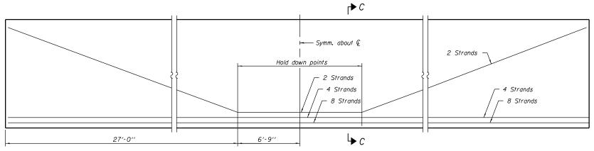
ELEVATION OF BEAM (Showing prestressing steel)
