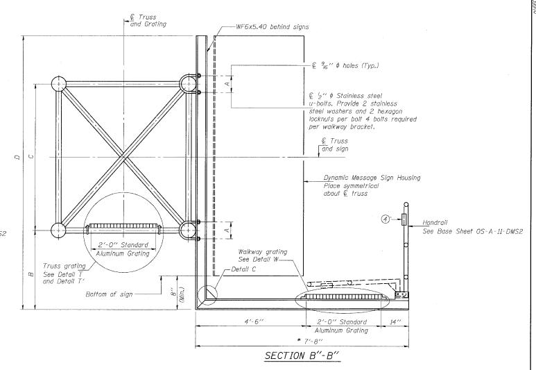
\* Bracket and grating dimensions are nominal and will vary based on actual DMS cabinet dimensions plus manufacturer's mounting devices, and providing clearance between the lowered handrail and DMS cabinet.
