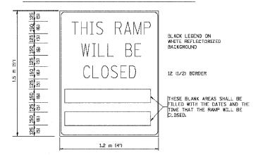
THESE SIGNS ARE REQUIRED ON BOTH SIDES OF THE RAMP, 4 MINIMUM OF 1 WEEK IN ADVANCE OF THE CLOSURE.
