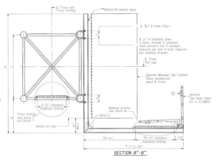
\* Bracket and grating dimensions are nominal and will vary based on actual DMS cabinet dimensions plus manufacturer's mounting devices, and providing clearance between the lowered handrail and DMS cabinet.
