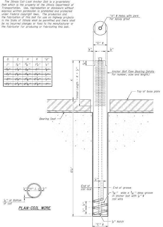
ILLINOIS COIL-LOCK ANCHOR BOLT
