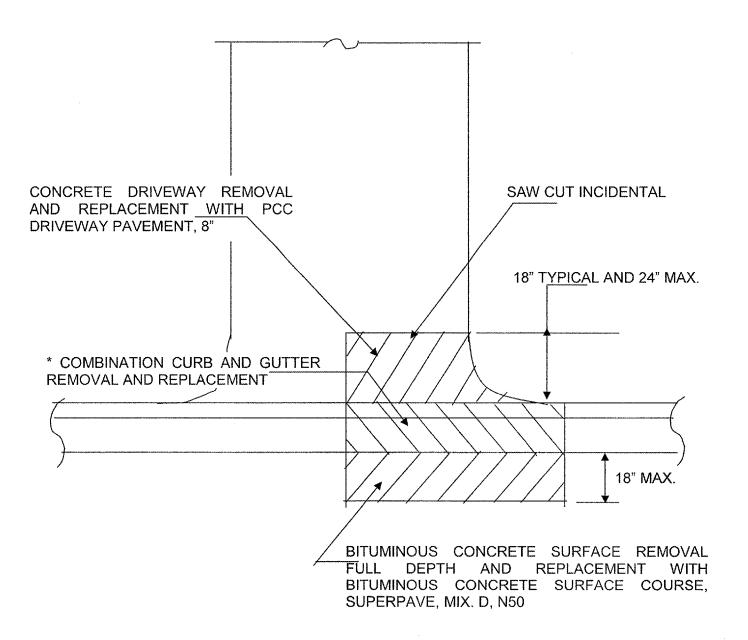
\* PROPOSED DEPRESSED CURB AND EXACT LENGTH SHALL BE DETERMINED IN THE FIELD BY THE ENGINEER (TYPICAL)
