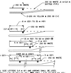
\* TURN LANES IN EXCESS OF 120 m (400°) IN LENGTH MAY HAVE AN ADDITIONAL SET OF ARROW - "ONLY" INSTALLED MIDWAY BETWEEN THE OTHER TWO SETS OF ARROW - "ONLY".
