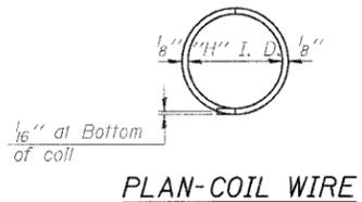
ILLINOIS COIL-LOCK ANCHOR BOLT
