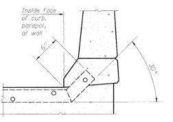
AT CURB, PARAPET, OR WALL (Showing plate)
