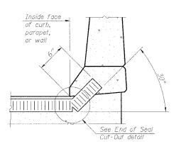
AT CURB, PARAPET, OR WALL (Showing seal)
