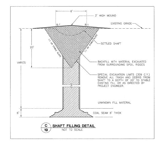
DUE TO THE UNKNOWN CONDITIONS THAT EXIST IN AND AROUND THE SHAFTS, THE CONTRACTOR SHALL USE EXTREME CAUTION WHEN PERFORMING WORK NEAR THEM. THE ENGINEER RESERVES THE RIGHT TO INCREASE OR DECREASE THE QUANTITY FOR SPECIAL EXCAVATION AND BACKFILLING MATERIALS AS DETERMINED BY THE EXACT CONDITIONS ENCOUNTERED DURING SPECIAL EXCAVATION.
