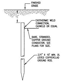
TYPE AND MINIMUM NUMBER OF GROUND RODS SHALL BE AS SPECIFIED ON THE PLAN.
