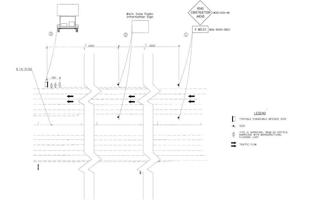
① THE ROAD CONSTRUCTION AHEAD SIGN SHALL BE LOCATED 3 TO 5 MILES IN ADVANCE OF THE PROJECT LIMITS,
