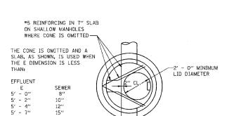
5' - 10" 18" NOTE: SEE SPECS. FOR FRAME COVER AND STEPS. MANHOLE STEPS SHALL BE PROVIDED TO
