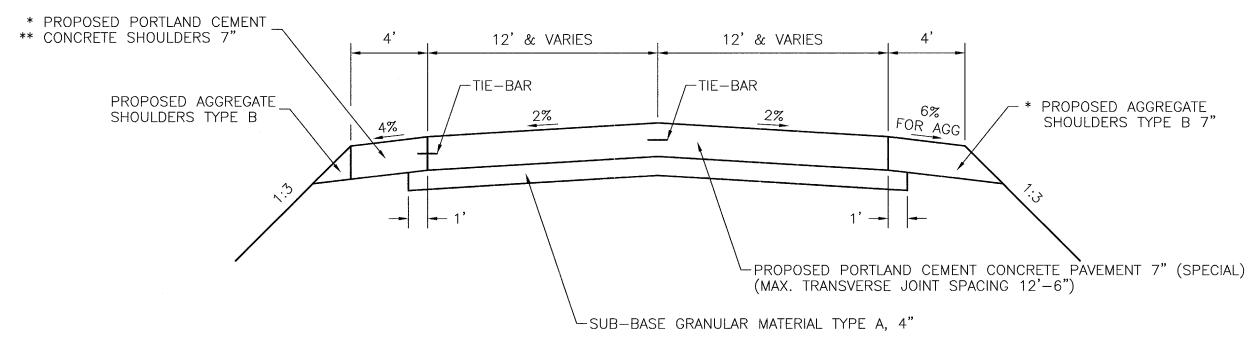
\* NOTE: SEE PLAN & PROFILE SHEETS FOR LOCATIONS OF PROPOSED PORTLAND CEMENT CONCRETE SHOULDERS & AGGREGATE SHOULDERS.
