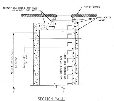
STANDARD MANHOLE BARREL
