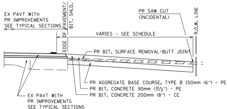
**SECTION A-A FOR EX BITUMINOUS PE & CE**
