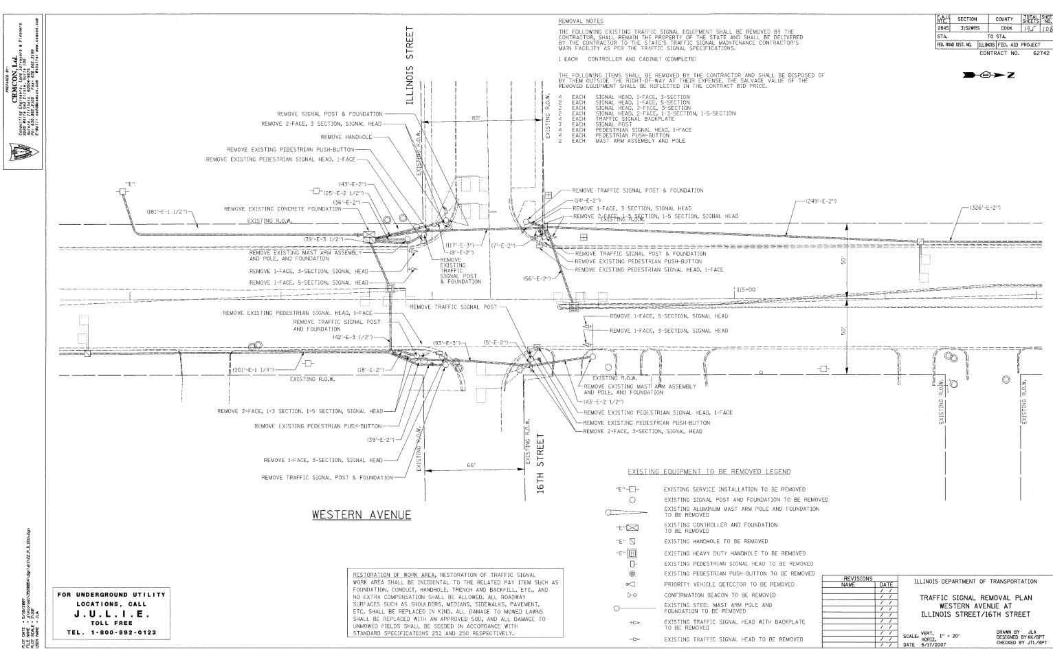
EXISTING TRAFFIC SIGNAL HEAD TO BE REMOVED
