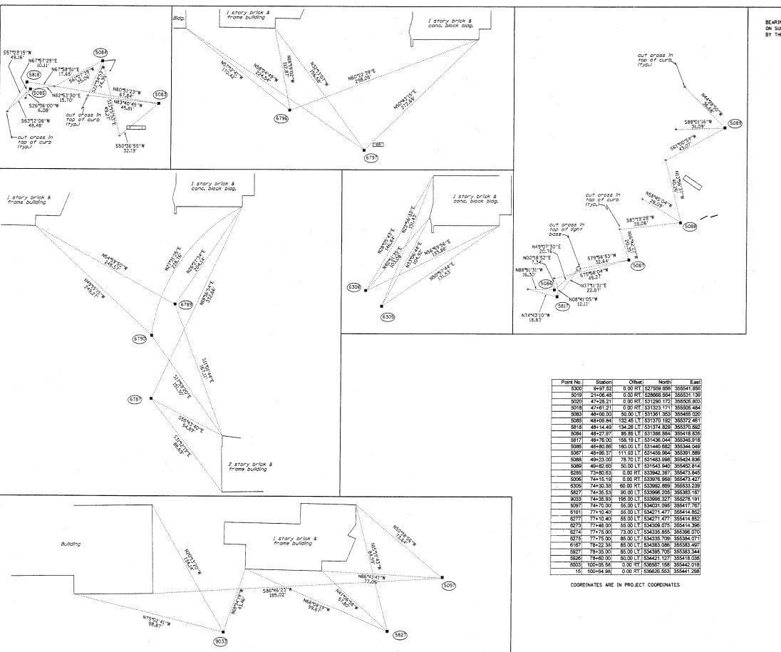
BEARINGS SHOWN HEREON ARE BASED ON SURVEY CONTROL DATA AS PROVIDED BY THE ILLINOIS DEPARTMENT OF TRANSPORTATION.
