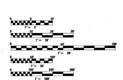
FULL SIZE PLANS HAVE BEEN PREPARED USING STANDARD ENGINEERING SCALES, REDUCED SIZED PLANS WILL NOT CONFORM TO STANDARD SCALES, IN MAKING MEASUREMENTS ON REDUCED PLANS, THE ABOVE SCALES MAY BE USED.
