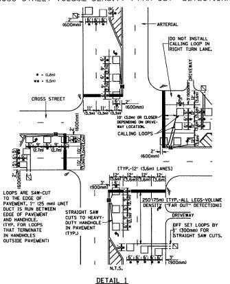
ARTERIAL-VOLUME DENSITY ("FAR OUT" DETECTION) CROSS STREET-NON VOLUME DENSITY ("UPTIGHT" PRESENCE DETECTION)
