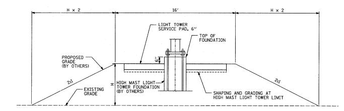
FILL GRADING DETAIL SECTION A-A
