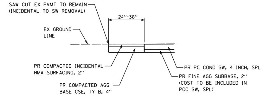
**DETAIL PR TIE TO EX PAVEMENT TO REMAIN
