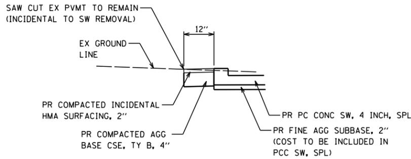
**DETAIL PR TIE TO EX PAVEMENT TO REMAIN
