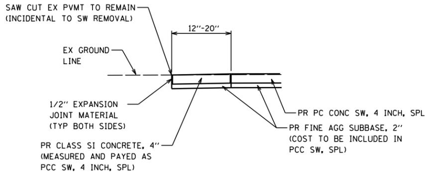
**DETAIL PR TIE TO EX PAVEMENT TO REMAIN
