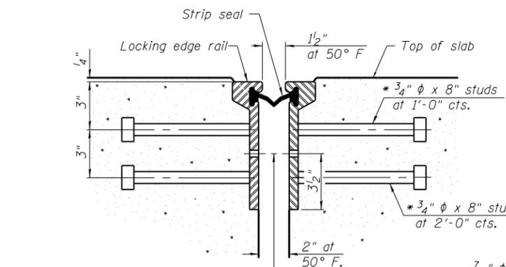
7/16"  $\phi$  holes at 4'-0" cts. for 3/8"  $\phi$  bolts. All bolts shall be burned, sawed, or chipped off flush with the plates after forms are removed, typ.
