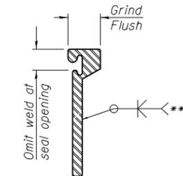
\*\*\* Back gouge not required if complete joint penetration is verified by mock-up.
