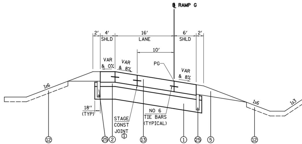
**PROPOSED RAMP G SUPERELEVATED SECTION**
