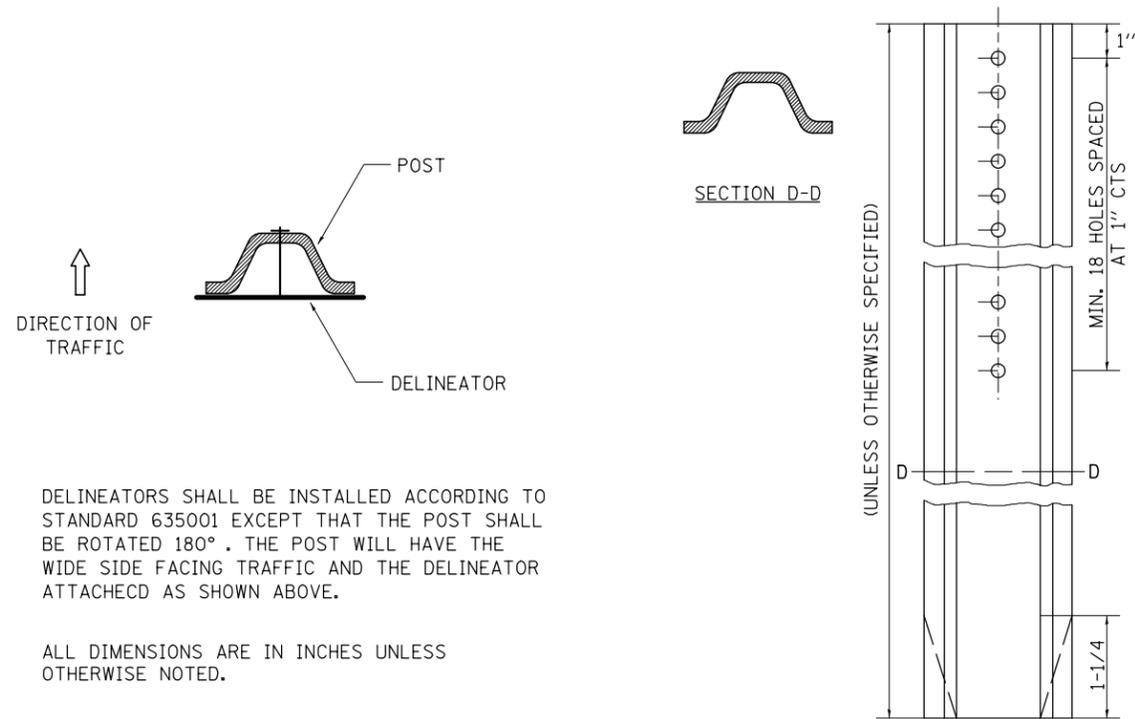
DELINEATORS SHALL BE INSTALLED ACCORDING TO STANDARD 635001 EXCEPT THAT THE POST SHALL BE ROTATED 180°. THE POST WILL HAVE THE WIDE SIDE FACING TRAFFIC AND THE DELINEATOR ATTACHED AS SHOWN ABOVE.
